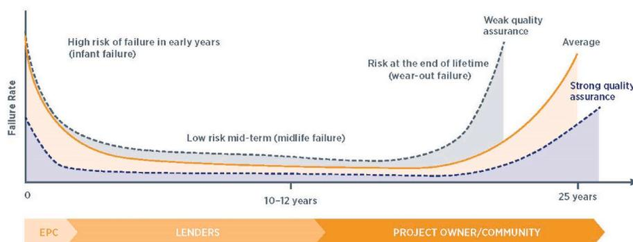
Fig. 2. Failure curve of a solar PV system, reprinted from Ref. [7], p.12.
