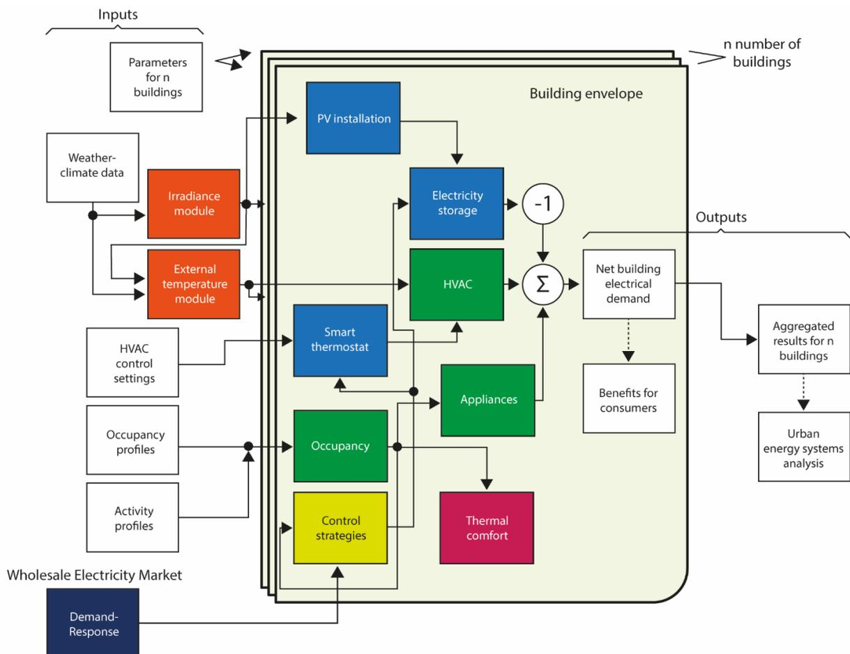
**Figure 4:** The DREEM model's architecture as it currently stands. Source: Stavarakas and Flamos, 2020.
