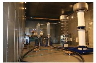
Fig. 6. Testing loop shown together with the 800 kV DC generator on the Nexans testing platform (courtesy of Nexans).
