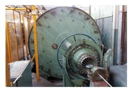
Fig. 3. Planetary cabling machine from Nexans used to manufacture the cable conductor for Best Paths (courtesy of Nexans).
