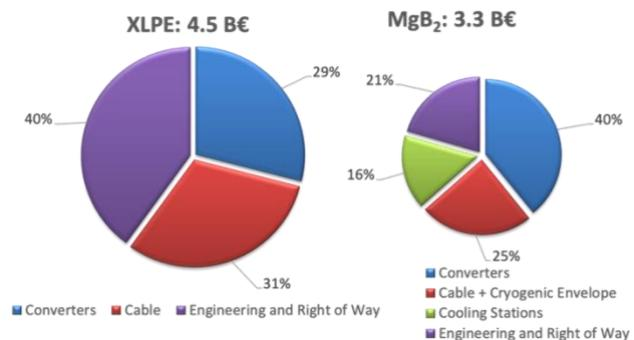
Fig. 7. Capital costs of resistive XLPE cables and MgB<sub>2</sub> superconducting cables for a 6.4 GW DC power link with a length of 500 km.
