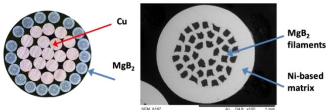
Fig. 2. Picture of the 10 kA cable conductor consisting of 18  $\text{MgB}_2$  wires wound around a copper core (left) and one  $\text{MgB}_2$  wire composed of 36 superconducting filaments embedded in a matrix of nickel and monel (right).
