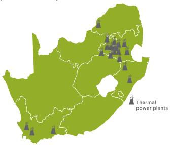
Figure 7: Location of thermal power plants (coal, diesel, and natural gas) in South Africa
